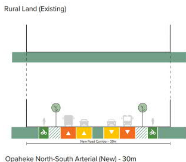
Figure 9-2: Ōpāheke North-South FTN arterial (NoR D4) future corridor design
