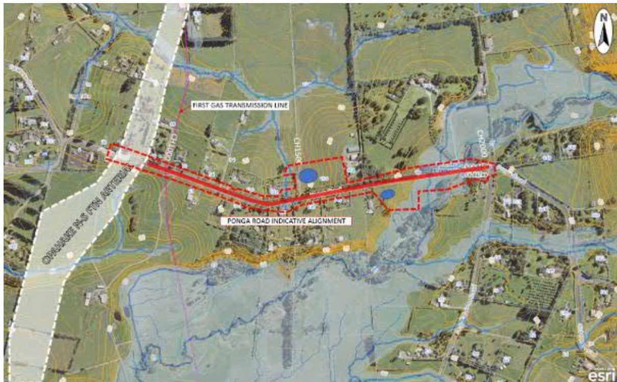
Figure 10-18: Extent of works - Ponga Road upgrade
