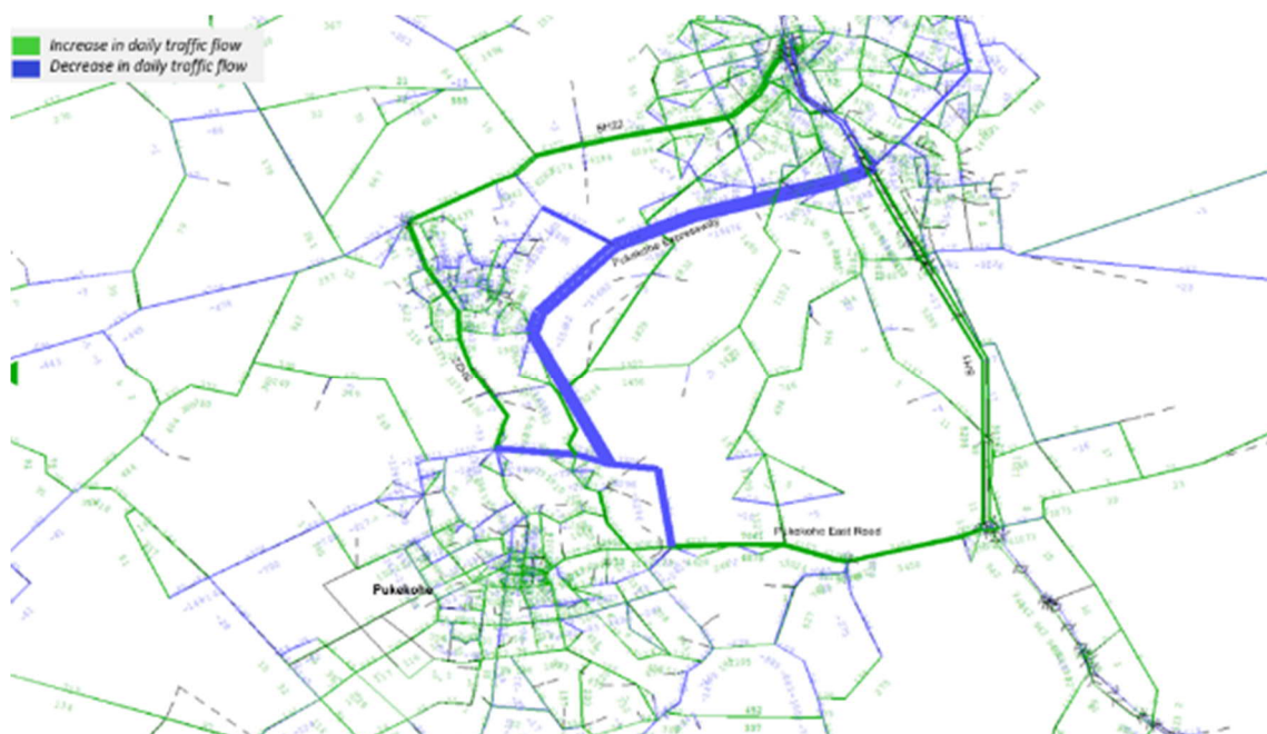
Figure 6-14: 2038 Rerouting Effect Without Pukekohe Expressway
