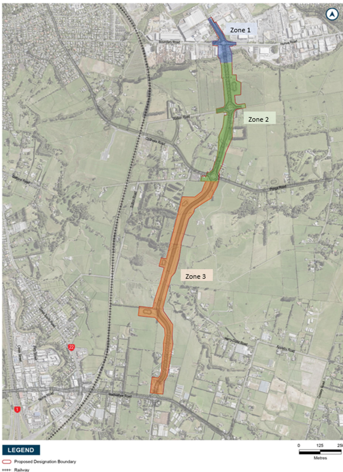
Figure 9-13: Construction zones – Ōpāheke N-S FTN Arterial
